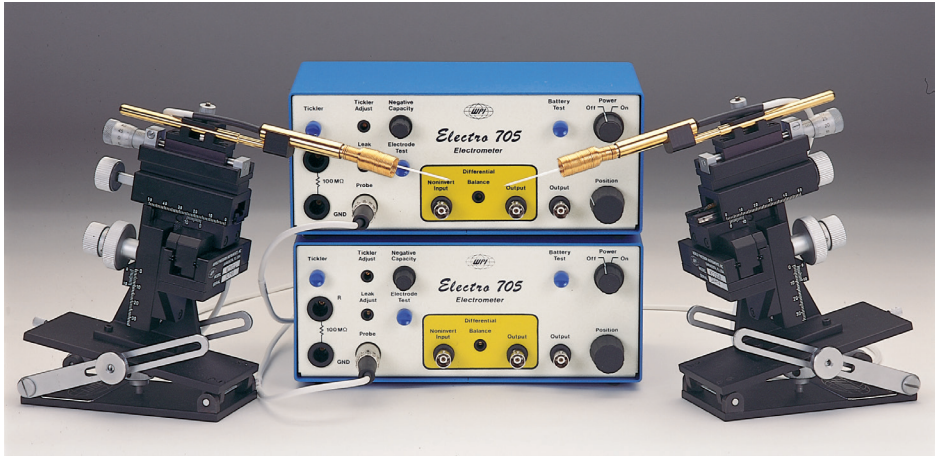
Fig. 1—Electro705 System. Two 705's can be linked together to form a high impedance differential electrometer pair.
